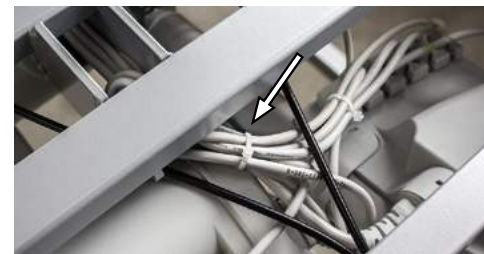
Position of the cable clip over the lying surface motor at the foot end .
