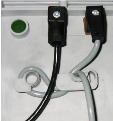
Routing the hand control cable
